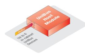
UniBus Devices are designed for installation within the same enclosure as the UniBus host module. A UniBus host can interface a maximum of six UniBus devices in any combination, provided they are all within the intended functionality of the host module
