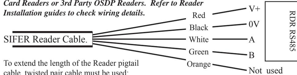
To extend the length of the Reader pigtail cable, twisted pair cable must be used:
