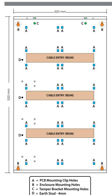
Figure 6: MW730B - Large Enclosure Details
