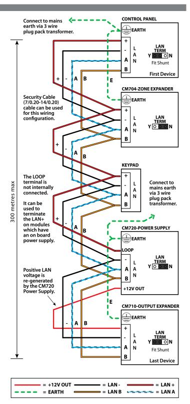
Figure 18: LAN Connection Using 2 Pair Security Cable
