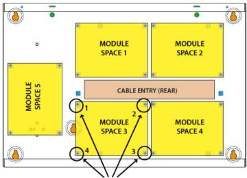
When installing small modules, you should fit 4 mounting clips as shown.
