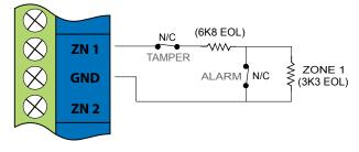
Figure 12: N/C Zone With Tamper
