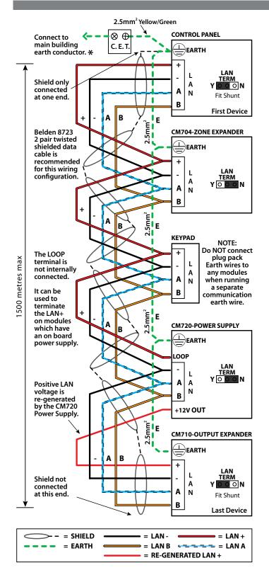
Figure 19: LAN Connection Using Twisted Pair Cable
