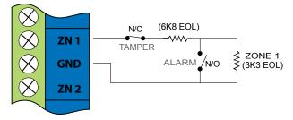
Figure 16: N/O Zone With Tamper
