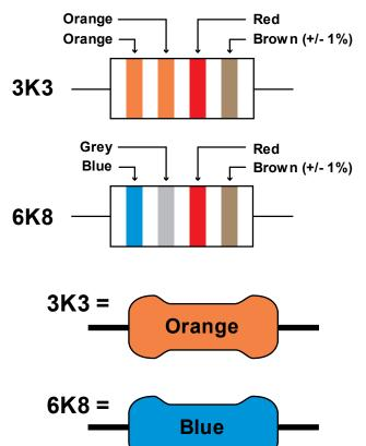
Figure 17: EOL Resistor Colour Chart
