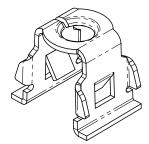
Figure 4: PCB Mounting Clip
