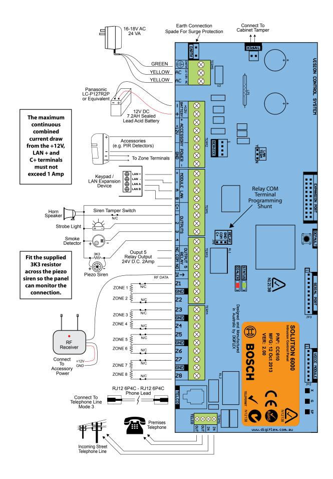
Figure 21: Solution 6000 Connection Diagram
