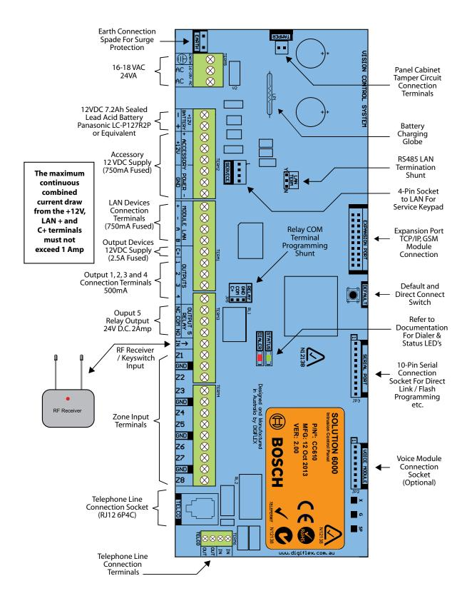
Figure 20: Solution 6000 Board Layout
