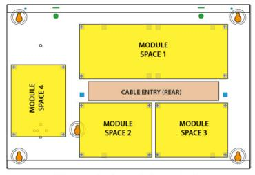
When installing large modules, you should fit 5 mounting clips as shown.
