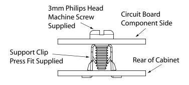
Figure 1: PCB and Mounting Clip Installation Diagram
